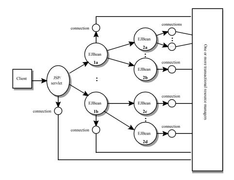
Figure EE.4-1 Servlets/JSP Pages Accessing Enterprise Beans
