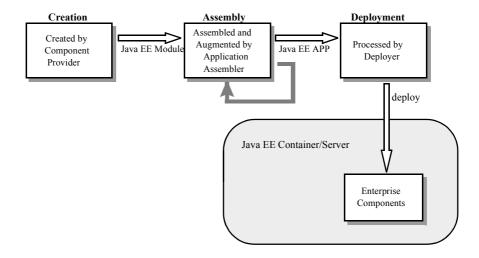
Figure EE.8-2 Java EE Application Life Cycle
