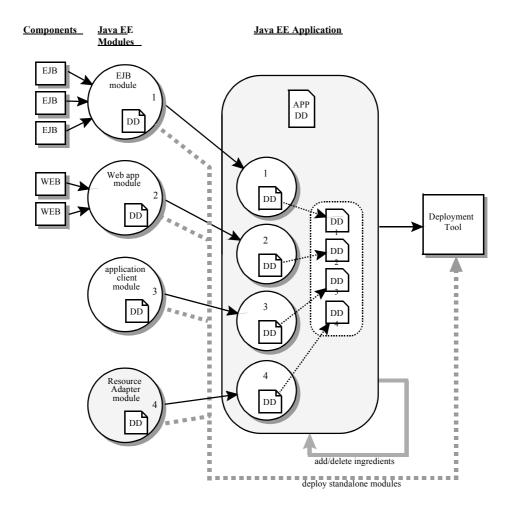
Figure EE.8-1 Java EE Deployment
